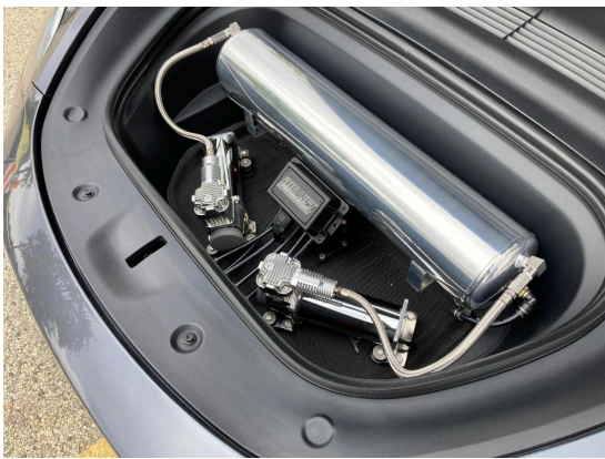
Air suspension tank in the frunk - Model 3
