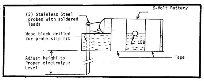
In use, the probes are adjusted so the tips are at the correct electrolyte level for a cell. The BELL body is then placed on the battery with probes extending into the cell. Distilled water is then added until the LED is illuminated by completing the 9-volt circuit through the electrolyte.
