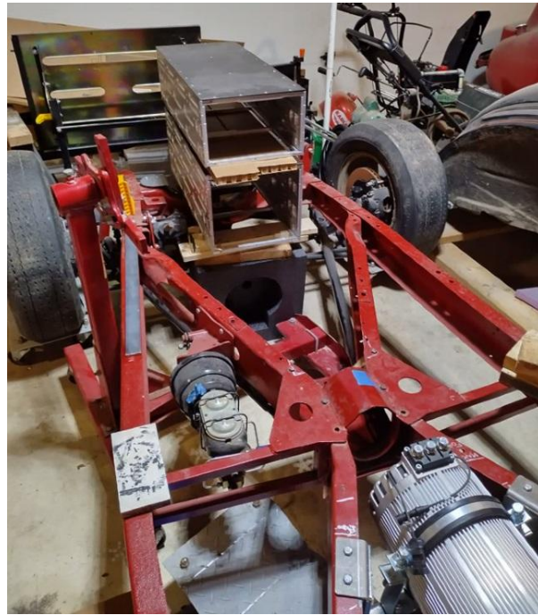
Looking towards the front, w the location of the two stacked battery boxes
