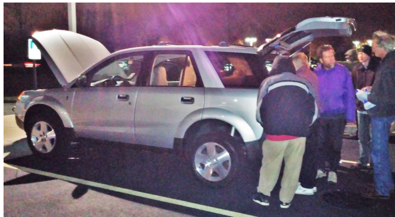
Steve's Saturn Vue conversion has 70,000 electric miles over the last 7 years. SUV Range is 95 electric miles using 172V battery pack made up of 45 Thundersky 200Ah Cells. Steve appreciated the excellent work of John Emde, Rich Carroll, John Jeidi, Ted Lowe and Rich Grushas in converting this SUV to electric. Wow great work everyone!! Thanks Steve for sharing your experience with a pioneering electric vehicle.
