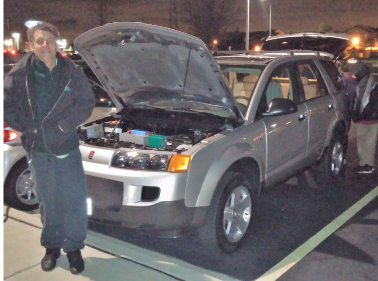
Steve's Saturn Vue conversion has 70,000 electric miles over the last 7 years. SUV Range is 95 electric miles using 172V battery pack made up of 45 Thundersky 200Ah Cells. Steve appreciated the excellent work of John Emde, Rich Carroll, John Jeidi, Ted Lowe and Rich Grushas in converting this SUV to electric. Wow great work everyone!! Thanks Steve for sharing your experience with a pioneering electric vehicle.
