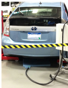
Testing Wireless Charging
