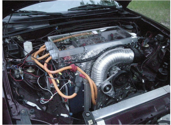
The Miata custom electric motor configuration that George Hiller created
